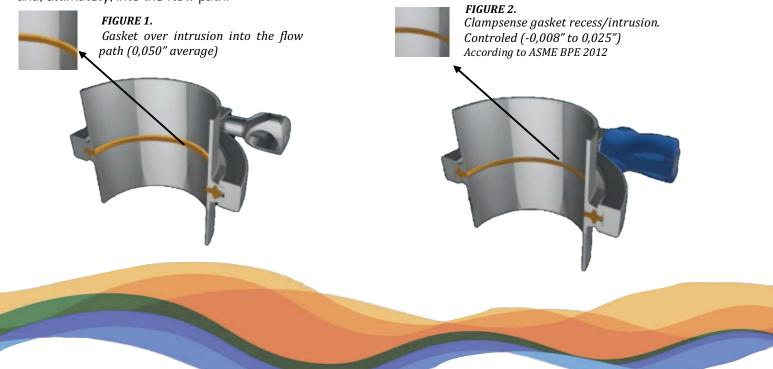
Figure 1 shows how the intrusion disturbs product flow. Even when the CIP solution, a pipe cleaning solution, flows through the system it becomes clearly evident that the space beneath the intrusion is not being cleaned properly.
